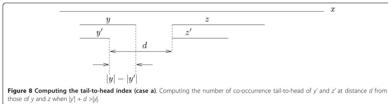
**Figure 8 Computing the tail-to-head index (case a).** Computing the number of co-occurrence tail-to-head of  $y'$  and  $z'$  at distance  $d$  from those of  $y$  and  $z$  when  $|y| + d > |y'|$ .
