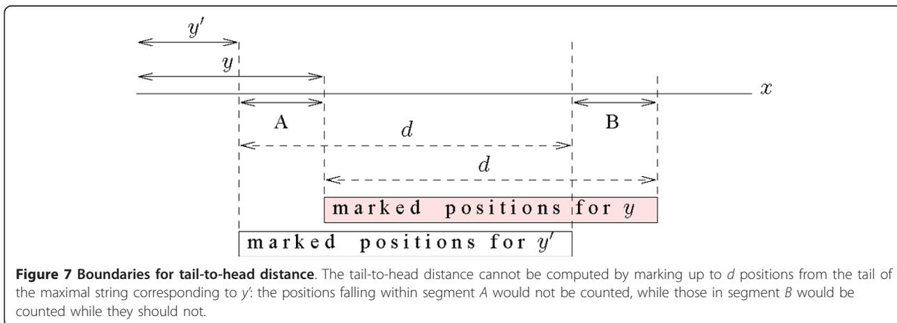
**Figure 7 Boundaries for tail-to-head distance.** The tail-to-head distance cannot be computed by marking up to  $d$  positions from the tail of the maximal string corresponding to  $y'$ : the positions falling within segment A would not be counted, while those in segment B would be counted while they should not.
