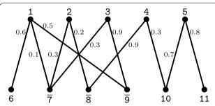
**Fig. 2** Example of similarity graph. Here we show the graph  $S_{0,1}(A,B)$  for the two genomes  $A = \{[1\ 2\ 3\ 4\ 5]\}$  and  $B = \{[6\ \overline{7}\ \overline{8}\ \overline{9}\ 10\ 11]\}$
